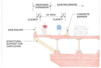
Figure 54c. The pedestrian way across the bridge could be added and retrofitted into the existing bridge infrastructure.
